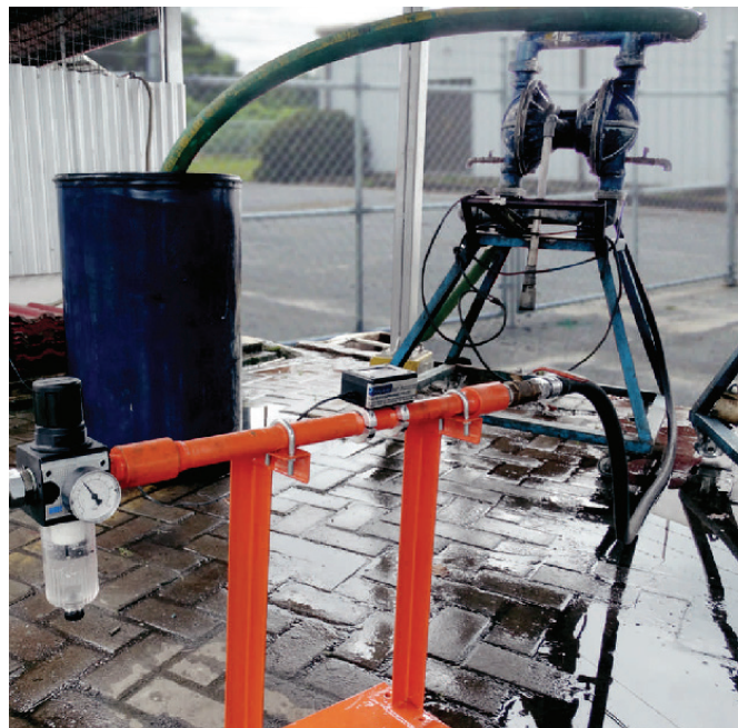
An on-site, head-to-head test at the IndoChem facility unequivocally that a Wilden SHIFT ADS shortened the loading time while cutting air consumption (competitor pump shown).
