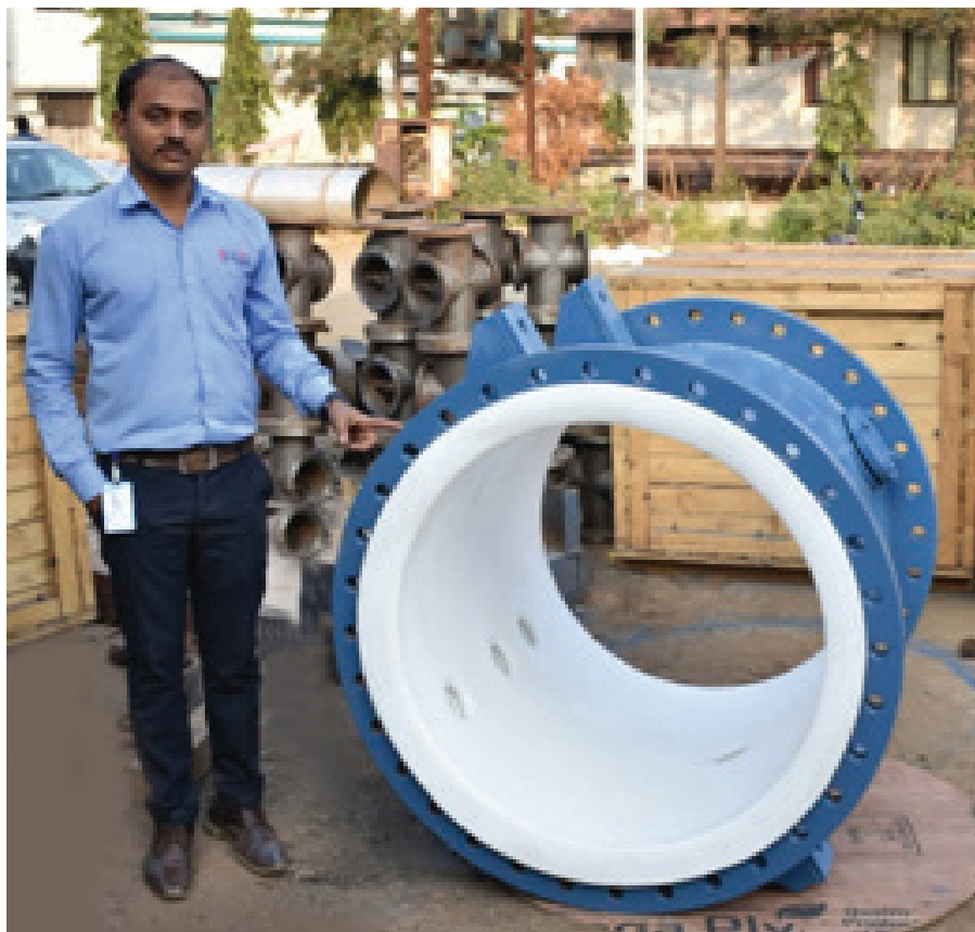
36 inch dia. PTFE lined equipment for corrosive chemical handling.
