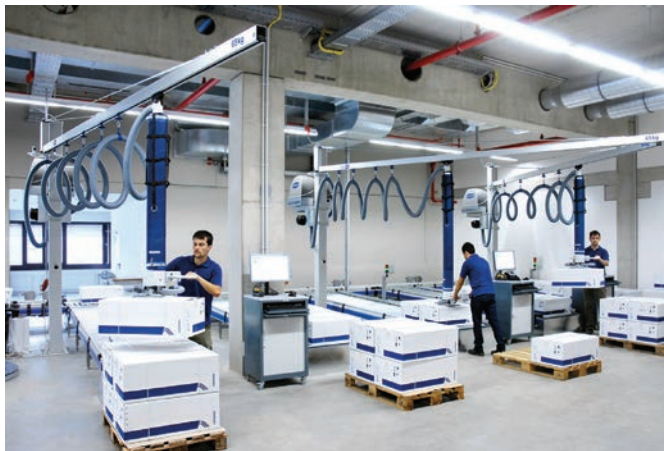
Efficient yarn handling in textile mills with vacuum tube lifters jumbo
